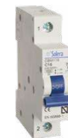
Magnetotérmico estreito Solera 1 polo 10A Ref. 02863 16A Ref. 02864 20A Ref. 02865 25A Ref. 02866 32A Ref. 02867 40A Ref. 02868
